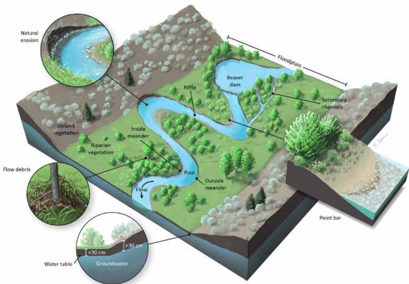
Figure 2. This illustration depicts key features of a functional stream, such as beaver dams, gently sloped point bars with riparian plants establishing, natural erosion occurring on the outside bends of stream meanders, evidence of bank overflow shown by flow debris captured on the upstream side of trees/shrubs and a depth to water table throughout the floodplain that is 30 centimeters or less and capable of sustaining native riparian vegetation. Upland vegetation typically occurs outside of the floodplain. The stream meanders through the entire floodplain. Additional components of stream systems often include secondary channels, pools that are deeper than the rest of the channel and riffles where more shallow water flows over the stream's substrate.
