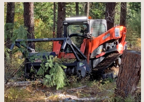
Masticators grind up small trees and underbrush.
