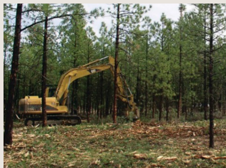
Mastication with an excavator with grinding head. Photo: Steve Fitzgerald.
