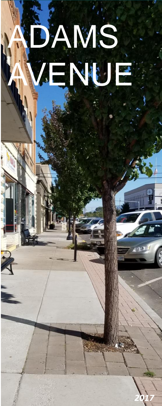
Figure 1. The generously sized tree wells offer trees 50 cubic feet of soil volume.
